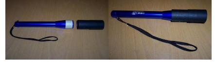
This technique for making an LED flashlight work as a pointer can be applied to other brands and makes of LED flashlights. You just need to adjust the dimensions of the cylinders and diameters of the lens and lens mask to fit your flashlight.
