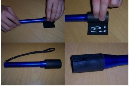
2. Wrap the 1  $\frac{1}{2}$  in. X 6 in. piece of railroad board around the *Focus Cylinder* (#1) and roll it gently. Leave a little space at the end to apply your choice of hot glue or white glue/clear tape. Then continue rolling so that the glue adheres. If you use white glue you will need to hold the cylinder closed with clear tape. This is the *Cap Cylinder* (#2).
