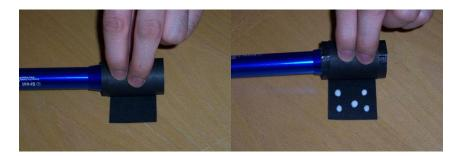
3. Remove the Focus and Cap cylinders from the flashlight head and wrap the <sup>3</sup>/<sub>4</sub> in. X 6 in. piece of railroad board around the head of the flashlight and roll it gently. Leave a little space at the end to apply your choice of hot glue or white glue/clear tape. Then continue rolling so that the glue adheres. If you use white glue you will need to hold the cylinder closed with clear tape. This is the *Lens Cylinder* (#3).
